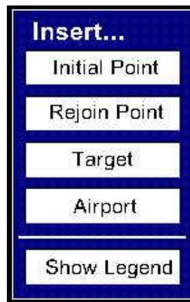
Fig. 4.2: Typical action window on the digital map table. The example shows the action window for the crosshairs marker.
